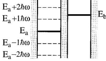
FIG. 1. The two-level double quantum-well system with the relevant virtual states.
